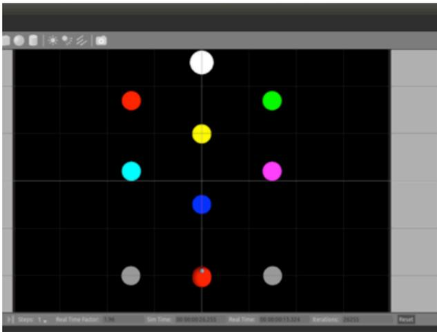
Figure 1: Gazebo robot simulator. Screenshot of Gazebo simulator showing the prototypical top view of a foraging task used to benchmark DAC with colored patches on the floor and a source of light represented by a bigger white patch on top of the screen.
