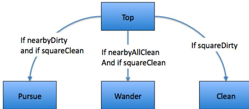
Figure 7 – The problem space hierarchy used by CleaningTom the vacuum cleaner.
