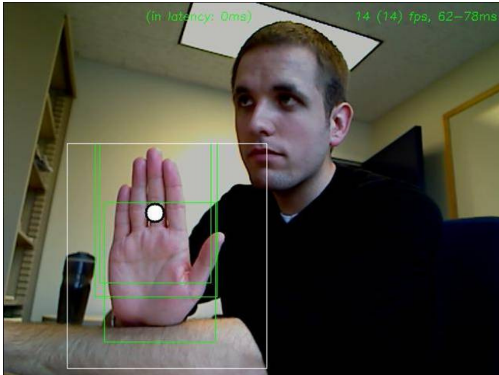
Figure 2: The "Closed" Hand Posture Being Recognized by HandVu
